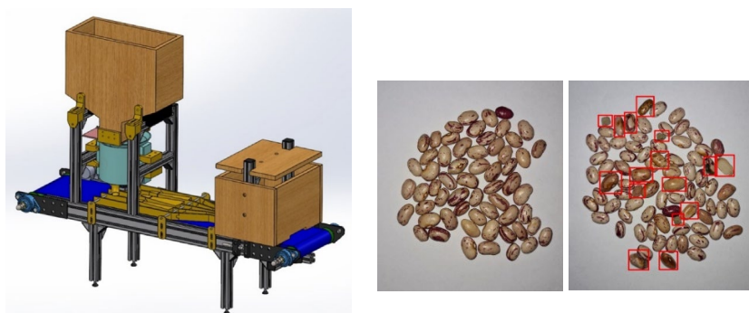
Figure 15: CAD model of the sorting system and examples of defective bean grains.
