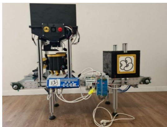
Figure 16: Final fabricated prototype of the bean grain sorting machine.
