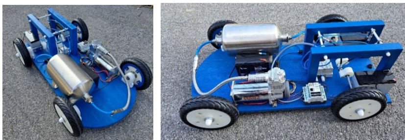
Figure 2: Autonomous vehicle actuated by PAMs.
