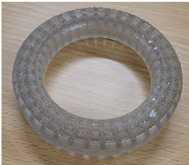
Figure 5: 3D printed elastic buffer.
