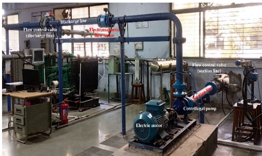
Figure 1: Centrifugal pump test setup.
