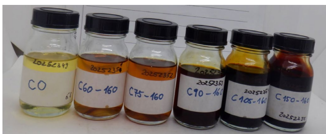
Figure 4: Colour changes as a result of thermal stress in case of sample C.
