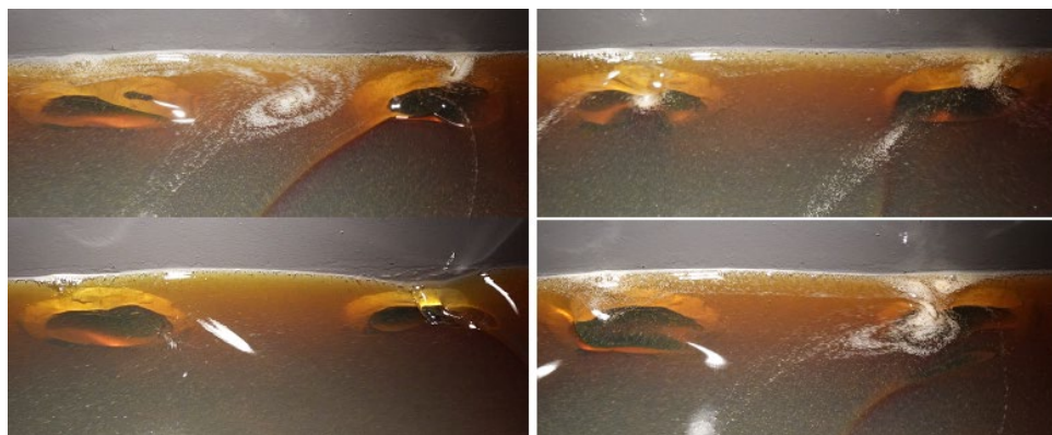
Figure 12: Pumping air from the surface into the suction lines – view of the tank from above.
