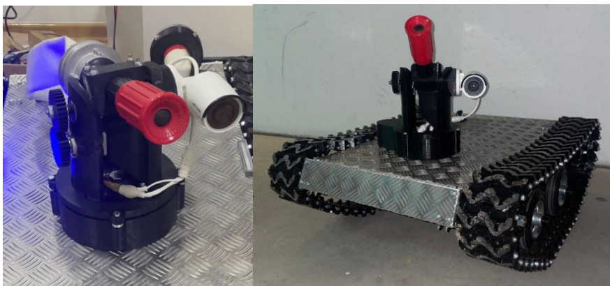
Figure 4: Mobile fire-fighting robot with mounted rotating turret.
